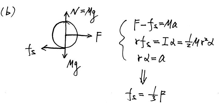
$F_{net} = F - f_s = \frac{2}{3}F = \frac{2}{3}(-kx)$  $\therefore \quad \mathcal{A} = \frac{F_{net}}{M} = -\frac{zk}{3M}X \implies \qquad \ddot{X} = -\frac{zk}{3M}X$  $W = \sqrt{\frac{2k}{3M}}, \quad T = \frac{2\pi}{W} = 2\pi \sqrt{\frac{3M}{2k}}.$ If you plug in the numerical value for k you should get  $T = 2\pi \sqrt{\frac{4}{5}} = 4.44 \sqrt{\frac{4}{5}}$
