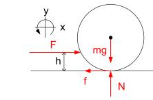
We use F = ma and  $\tau_{CM} = I_{CM}\alpha$  to find the linear and rotational acceleration. Since they are both constant, we can use the basic kinematics formulas to find the velocities.
