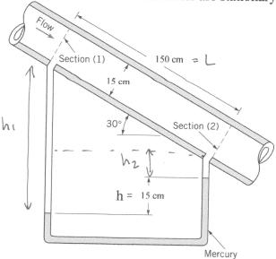
a) Find the pressure difference (P<sub>1</sub>-P<sub>2</sub>) between sections 1 and 2. (5 points)
