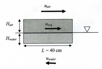
Floating raft -> weight balances buoyancy
