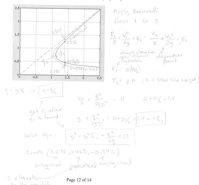
b) Suppose the channel now transitions from a width of  $b_1 = 2$  m to  $b_2 = 3$  m. Calculate the new alternate depths are and show which one will be chosen depending on the choice of upstream depth (i.e. you should have two answers and two explanations). The roots to your new cubic equation are (1.350, 0.285, -0.235). Label these on your diagram above. (10 points)
