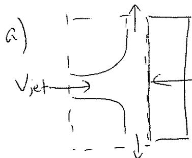
$$\sum F_x = \dot{m} V_{out} - \dot{m} V_{in}$$
