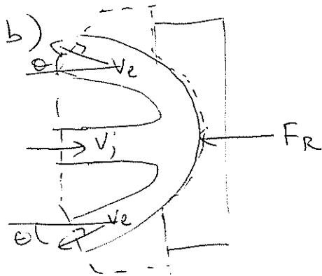
$$\sum F_x = \dot{m} V_{out} - \dot{m} V_{in} \quad \leftarrow V_{out,in} \text{ must be in } x \text{ direction}$$
