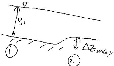
The max allowable step size for this flow rate is  $\Delta z_{\max}$  which will make the flow critical over the bump.
