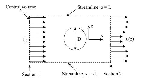
a) Use the setup shown above to perform a momentum balance for a cylinder of height H (into the page) using the control volume shown to find an analytical (integral) expression for the drag force exerted on the bridge pier. In which direction does the drag force act? (15 points)
