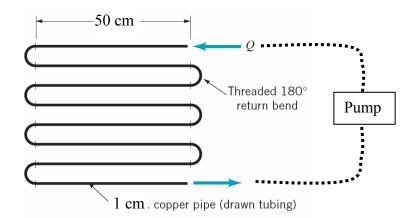
a) First calculate the Reynolds number through the pipe and decide if the flow is laminar or turbulent. Determine the friction factor for flow through the pipe. (5 points)
