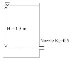
c) Now consider the flow when a 50 m long pipe is connected to the reservoir after the nozzle, as drawn below. The diameter of the pipe is 25 mm. Assume the pipe has an equivalent roughness of 0.5 mm. What is the new volume flow rate exiting the pipe? (8 points)
