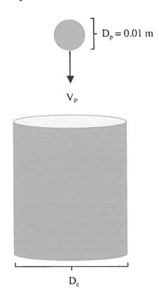
a) Calculate the initial terminal velocity of the ball before it reaches the cylinder. Check any assumptions you make. Circle your answer.
