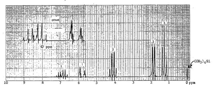
Integration, chemical shifts, multiplicities, assignments of absorptions. The spectrum is reported as follows:  $\delta = 1.24$  (t, J = 6.8 Hz), 1.88 (dd, J = 6.8, 1.7 Hz), 4.13 (q, J = 6.8 Hz), 5.81 (dq, J = 16.0, 1.7 Hz), 6.95 (dq, J = 16.0, 6.8 Hz).
