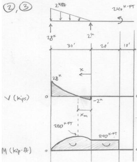
shear diagram: use  $\frac{dV}{dx} = -w$
