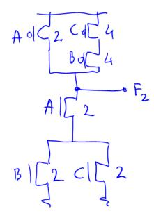
(c) [4pts] For 251A students only: Which 2-input Boolean logic function does the circuit below represent? Make sure to simplify the Boolean expression to the Boolean function you can recognize.
