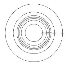
Lines with arrows are field lines for  $\vec{B}$ . The field is stronger closer to the surface of the wire, both from inside and from outside
