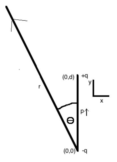
Figure 1: Diagram of dipole for Problem 2
