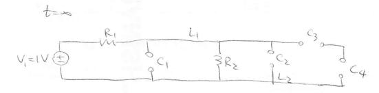
c) Since real capacitors have a leakage resistance, let's add that in. Consider the circuit below. (5 points)
