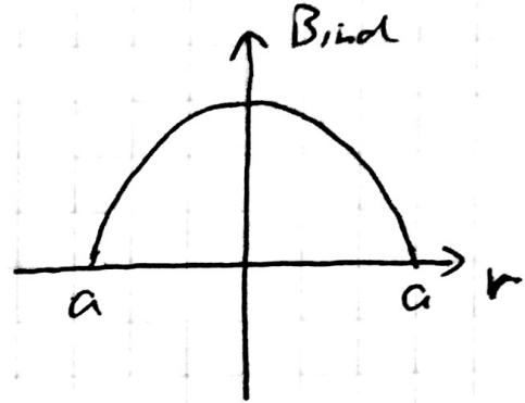
$$B_{\text{tot}} = B_{\text{solenoid}} + B_{\text{bind}}(r)$$
