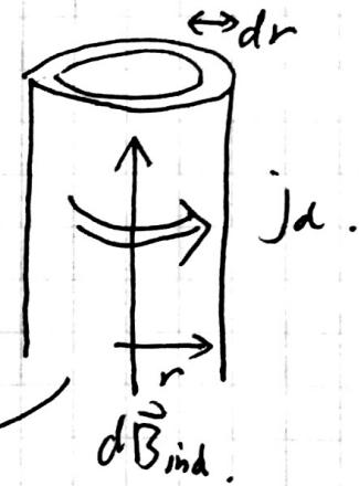
$$B_{\text{ind}} = \int_0^a d\vec{B}_{\text{ind}} = \frac{1}{2} \mu_0 n I_0 \frac{\omega^2}{c^2} \sin \omega t \int_0^a r dr .$$
