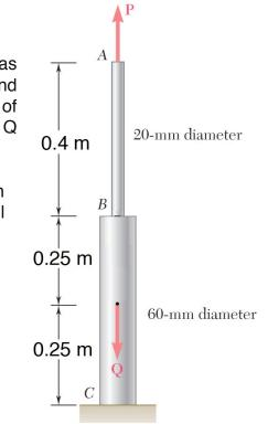
B) **5 pts** Determine the strain in rod portion AB. Be sure to specify if it is tensile or compressive.
