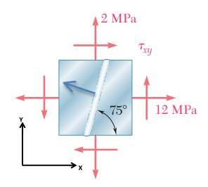
B) **10 pts** At this value of  $\tau_{xy}$ , what is the value of the normal stress acting perpendicular to the plane of the weld, *i.e.* along the direction of the normal vector shown above? Be sure to denote whether that is a tensile or compressive stress.
