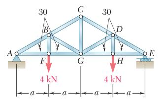
B) **15 pts** Determine the magnitude of the force in truss *EH* and also state whether it is in tension or compression.
