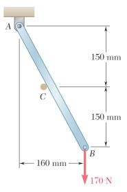
b- <u>Using equilibrium equations</u>, determine the magnitude of the contact force at C. **(10pts)**
