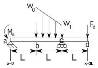
a- Determine the magnitude and x-location of the resultant force **R** for the distributed loading. **(15 pts)**
