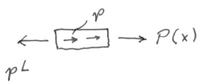
$$\begin{aligned} \sum F_x = 0 &= -PL + \int_0^x p dx + P(x) \\ &= -PL + px + P \Rightarrow \underline{\underline{P = p(L-x)}} \end{aligned}$$
