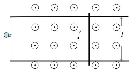
a. The rod is pushed at a constant velocity, v, so that the light bulb glows at 4.0 W. What is this velocity? You can neglect the resistance of the rails, and the resistance of the light bulb is 4.0  $\Omega$ .
