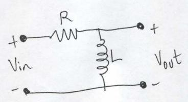
g) If  $v_{in}$  is a DC source equal to 1 V, what is the steady-state value of  $v_{out}$ ?
