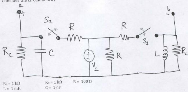
Switch 1 (S1) is closed (i.e. horizontal in the circuit above) for t < 0. Switch 2 (S2) is open (i.e. raised and not connected) for t < 0.
