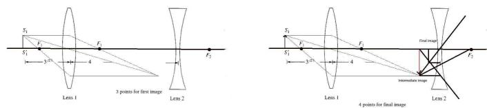
ii) Use the lens equation with a real object and a converging lens to find the initial image, which will serve as the object (caution! pay attention to the separation of the lenses) for the second lens.
