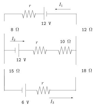
Answer: This is particularly simple as r = 1 and only reduction straight forward is series where  $R_{eq} = R_1 + R_2$ . One can reduce them further for purposes of solutions by recognizing some interchanges do not affect the other loops. E.g. the top loop where one can add the 12 $\Omega$  resistor to the series mix by a simple interchange.  $R_{top} = 12 + 1 + 8 = 21\Omega$  $R_{middle} = 1 + 10 = 11\Omega$  and the bottom loop  $R = 18 + 15 + 1 = 34\Omega$  In the end one
