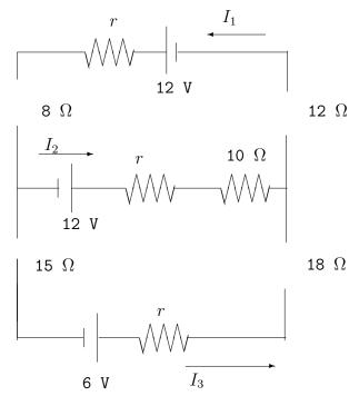
(b) [5 points] Write the appropriate equations and solve for the currents  $I_1$ ,  $I_2$ , and  $I_3$ .
