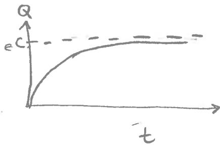
(b)  $I(t) = \frac{dQ}{dt} = \frac{EC}{RC} e^{-t/RC} = \frac{E}{R} e^{-t/RC}$
