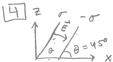
$$\text{Gauss: } |E_{in}| = 4\pi k \sigma$$
