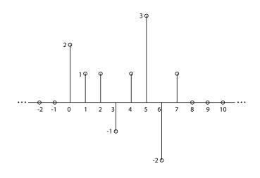
Given a discrete time sequence x[n] shown above (note x[n] is non-zero only for  $0 \le n \le 7$ ):
