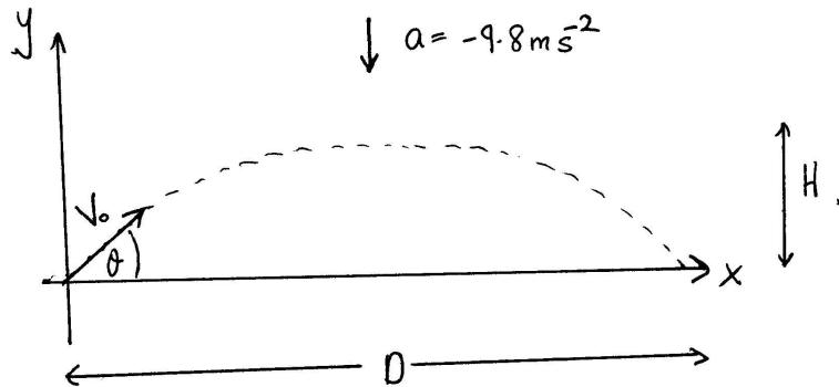
Given  $D = 9.0 \text{ m}$   $V_{0x} = 9.5 \text{ ms}^{-1}$
