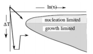
Grain boundaries are the result of uneven growth when the solid is crystallizing Grain boundaries are defects so they tend to decrease the electrical and thermal conductivity of the material. The free energy associated with forming a nucleusa=volume\*free energy (which is negative for transformation to happen) and surface area formation (which is always positive). Forming a surface always raises the energy.
