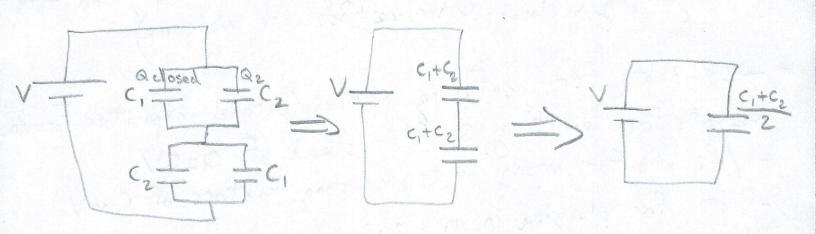
By symmetry, we can "guess"  $Q_{closed} = C, \bigvee$  from the first circuit since  $V_2'$  must be the voltage across each capacitor. Alternatively, proceed as before:  $Q_{total} = C_{eq}V = \frac{C_1+C_2}{2}V = 3C_2V$ .
