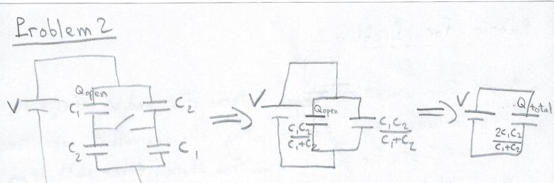
$Q_{total} = C_{eq}V = \frac{2C_{i}C_{2}}{C_{i}+C_{2}}V = \frac{2\cdot5C_{i}^{2}V}{6C_{2}}V = \frac{5}{3}C_{2}V$   $Q_{open} = \frac{1}{2}Q_{total} = \frac{5}{6}C_{2}V$
