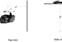
along the ground and travels a distance, d = 5 m, before stopping right at the edge of the cliff. The car flies off the cliff and after falling a height, H = 50 m, hits the ground, a distance, D = 30 m, from the bottom of the cliff. What is the coefficient of kinetic friction,  $\mu_k$ , between Young Kirk and the ground? Assume that the car did not slow down after Young Kirk dropped out of it.
