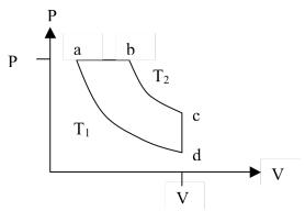
isothermal compression at temperature T<sub>1</sub>.
