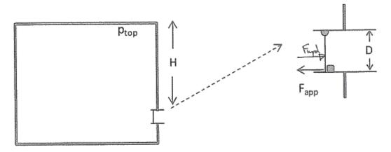
The pressure at the top of the tank, ptop = 49 kPa gage and the height of the tank from the top of the tank to the top of the gate is H=5 meters. The diameter of the outflowing pipe, which is cylindrical, is D=0.5 meters.
