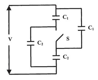
$C_1 = 5 \mu F$  and  $C_2 = 10 \mu F$
