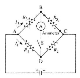
(a)(8 pts) Determine the relationship for  $R_x$  in terms of the known resistances  $R_1$ ,  $R_2$ , and  $R_3$  when the bridge is balanced.
