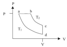
isothermal compression at temperature  $T_1$ .
