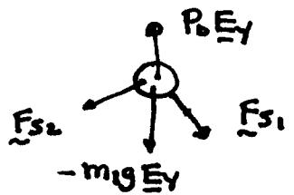
$$\underline{F}_{S1} = -K(||\underline{r}_1 - \underline{r}_2|| - l_0) \frac{\underline{r}_1 - \underline{r}_2}{||\underline{r}_1 - \underline{r}_2||}$$
