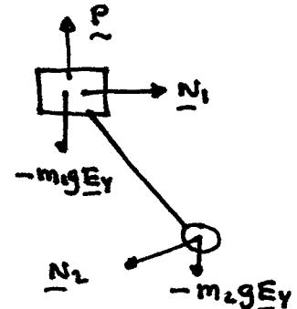
$$\underline{N}_1 = N_{1x} \underline{E}_x + N_{1z} \underline{E}_z, \quad \underline{N}_2 = N_{2z} \underline{E}_z$$
