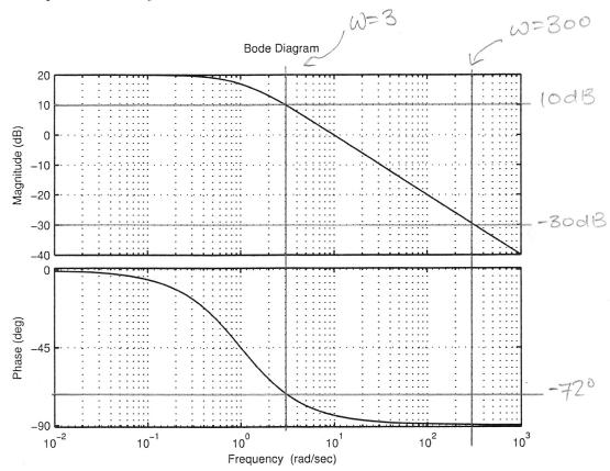
(a) Assume that the output has reached steady state after 4 seconds, based on the bode plot, draw the steady-state output  $y_{ss}(t)$  for  $\omega = 3$ . Make sure you label the response properly, i.e. amplitude, phase-shift, period.
