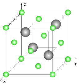
b. Ionically-bonded cesium chloride has Cl<sup>-</sup> at the center of a cube with Cs<sup>+</sup> at all eight corners. Alternatively, each Cs<sup>+</sup> ion is bonded to eight Cl<sup>-</sup> ions, also along the directions of the cube diagonals. Why is this not considered "directional" bonding?
