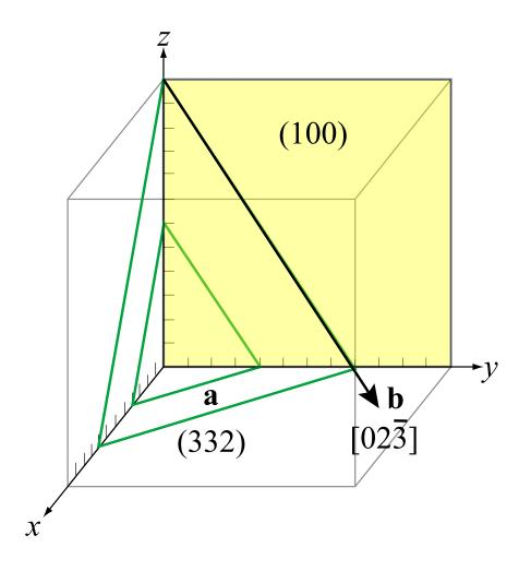
The (332) family is derived from fractional intercepts of  $\frac{1}{3}$  along the *x*-axis,  $\frac{1}{3}$  along the *y*-axis, and  $\frac{1}{2}$  along the *z*-axis, as **shown and labeled** on the drawing.
