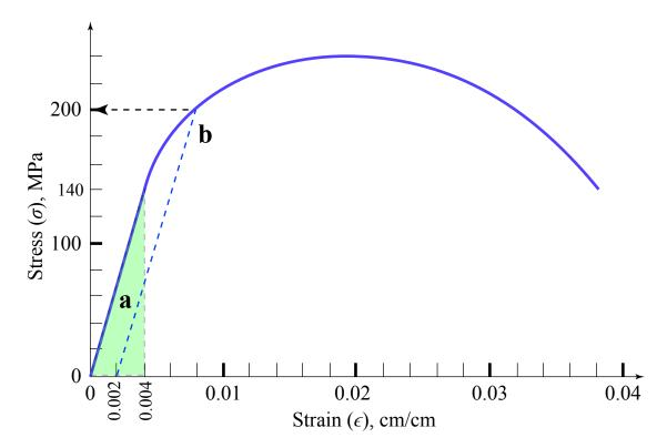
**a**. The specified elastic modulus for this component is "70 to 85 GPa." Does the alloy tested here fall within spec? Explain.
