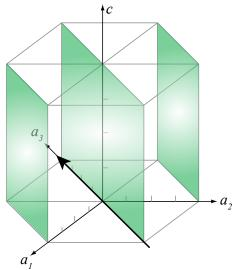
The line of intersection with the basal plane is fortuitously the  $a_3$  axis,  $[\bar{1}\bar{1}20]$ , which can also be expressed as its **negative**,  $[11\bar{2}0]$ . Either is correct.
