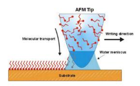
DPN is a direct-write scanning probe-based lithography. An AFM tip is used to deliver chemical reagents (peptides) to nanoscopic regions of a target substrate where they can self assemble. Desired chemistry is carried out exactly where it is needed.
