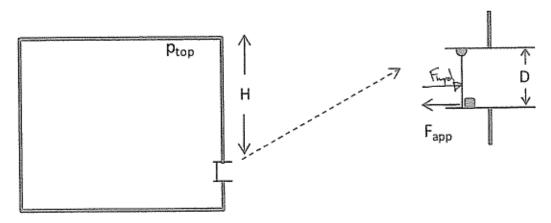
The pressure at the top of the tank, ptop = 49 kPa gage and the height of the tank from the top of the tank to the top of the gate is H = 5 meters. The diameter of the outflowing pipe, which is cylindrical, is D = 0.5 meters.
