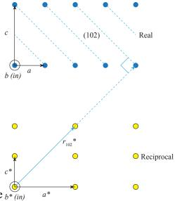
reciprocal lattice vector  $r_{102}^*$  is shown to be the normal to the (102) family of planes, with a magnitude equal to the reciprocal of the interplanar spacing. This is shown here by the relative magnitudes of  $a^*$ ,  $c^*$  and  $r_{102}^*$ .
