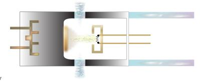
cause ionization of the target, triggering electronic transitions within the target to replace lost core shell electrons, generating **characteristic** x-rays with wavelengths specific to the energy levels of the target.
