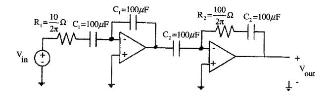
a. (15 pts) Let  $R_1 = 10/(2\pi)$  ohms,  $R_2 = 100/(2\pi)$  ohms,  $C_1 = 100$  uF, and  $C_2 = 100$  uF. Show that the transfer function of the circuit shown above is:
