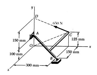
i) 10 pts Express the force as a 3D vector and determine its x, y, and z components.
