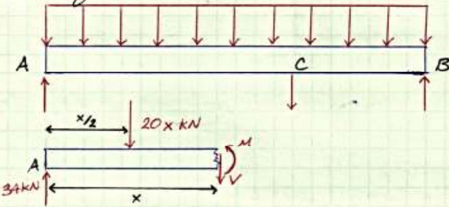
$$\sum F_y = 0 : 34 \text{ kN} - 20x \text{ kN} - V = 0$$
