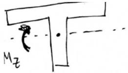
$$\sigma = \frac{Mc}{I} \quad \text{for max stress.}$$
