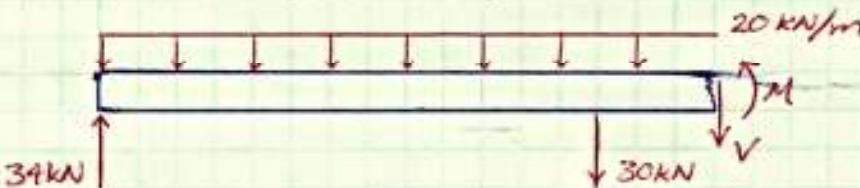
$$\sum F_y = 0 : 34 \text{ kN} - 30 \text{ kN} - V_{\text{dist}} - V = 0$$
