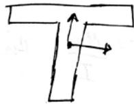
Break into sections and use the parallel axis theorem.
