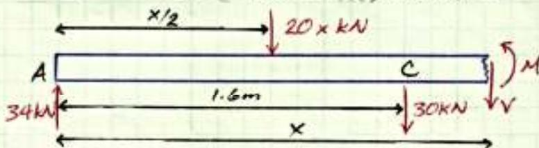
$$\sum F_y = 0 : 34 \text{ kN} - 20x \text{ kN} - 30 \text{ kN} - V = 0$$
