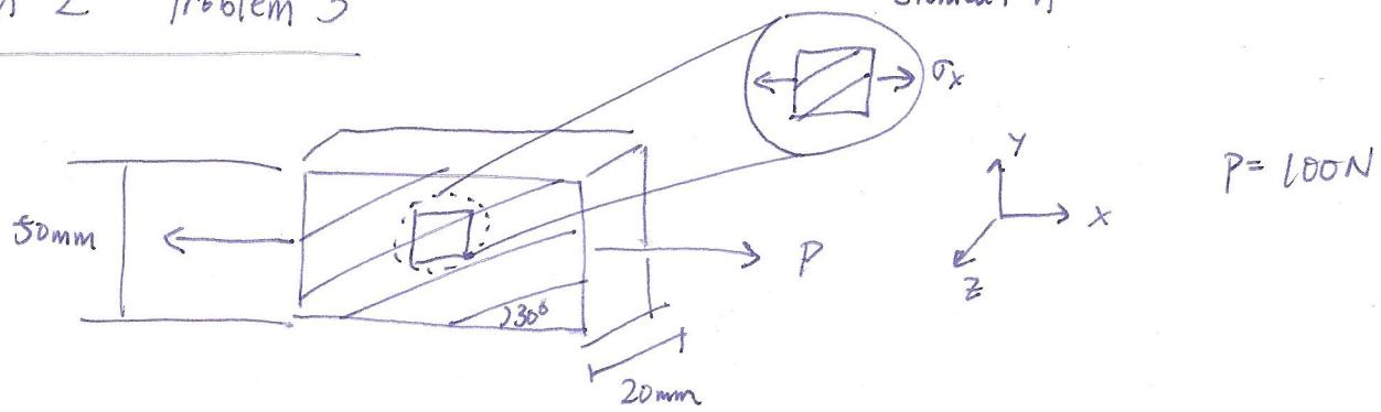
$$\sigma_x = \frac{P}{A_c} = \frac{100\text{N}}{(0.05\text{m})(0.02\text{m})} = 100000\text{Pa} = 0.1\text{ MPa}$$
