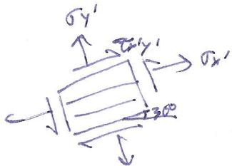
We see that  $\sigma_y'$  is the normal stress perpendicular to the grain.
