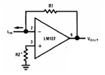
From Golden Rule #2, no current flows into or out of terminal V+. Then we know the voltage drop across R2 is zero. In turn, we know V + = 0.
