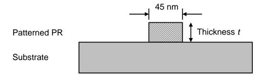
The profile above was created using a projection photolithographic method. The light source was an ArF excimer laser at 193nm.
