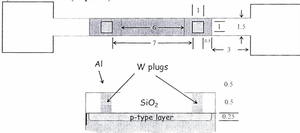
Calculate the resistance of this structure between the two large pads on either side. All dimensions are given in  $\mu\text{m}$ . Assume the p-layer is uniformly doped. Neglect current crowding effect (if you don't know what that is, don't worry about it). Use the following values:
