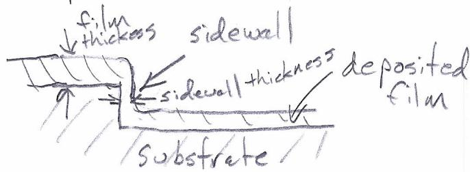
Step coverage is the ratio of the film thickness on the sidewall to the film thickness on the flat part of the wafer.
