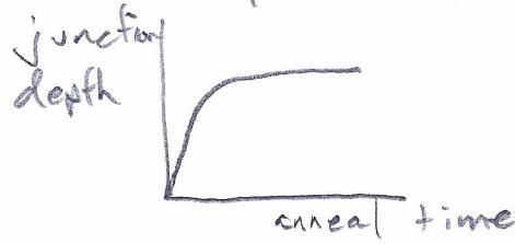
The plot shows the junction depth rapidly increases with anneal time at first, due to TED. After the defects anneal out, diffusion slows down.
