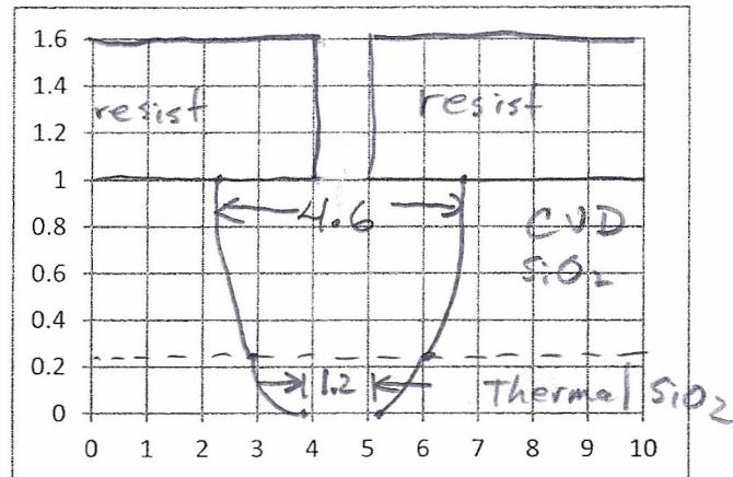
$0.75/0.3 = 2.5 \text{ min to etch CVD oxide. } 3.5 \text{ min overetch}$
