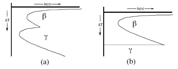
A one-component material has three possible structures,  $\alpha$ ,  $\beta$  and  $\gamma$ . At high T the system is  $\alpha$ . If it is cooled slowly it transforms to  $\beta$  at  $T < T_{\alpha\beta}$ , and remains  $\beta$  for all lower temperatures. If it is cooled quickly it transforms to  $\gamma$  at  $T_{\alpha\gamma} < T_{\alpha\beta}$ .
