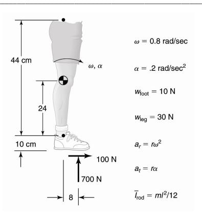
(i) [10 points] Draw a free body diagram for the combined femur-tibia rigid body. Draw another free body diagram for the foot. In both free body diagrams, include all accelerations.
