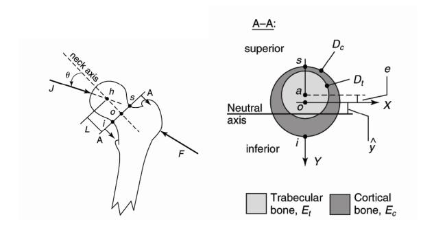
The stress acting on the inferior-most point, i, can be expressed by the following composite beam theory-based equation:
