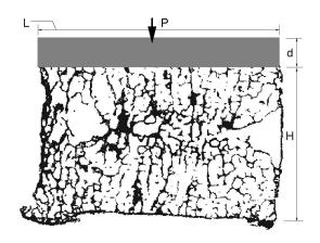
(i) [7 points] Derive the relationship between k (the "foundation modulus") and  $E_{TB}$  (the Young's modulus of the trabecular bone) in terms of the relevant dimensions. Assume that both the bone and the implant have a uniform depth b into the page.
