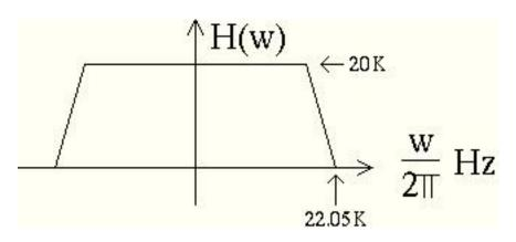
What is the standard (minimum) sampling frequency that is required for successful reproduction of any signal within that frequency band?
