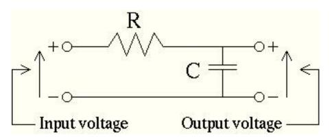
(1) Derive the frequency response *H-RC*(omega) of this filter.
