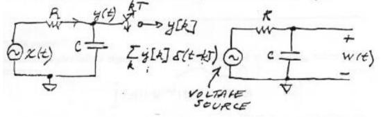
a. Find the transfer funciton of the continuous-time system from input x(t) to output y(t).
