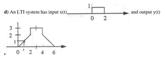
The output for an impulse input is sketch:
