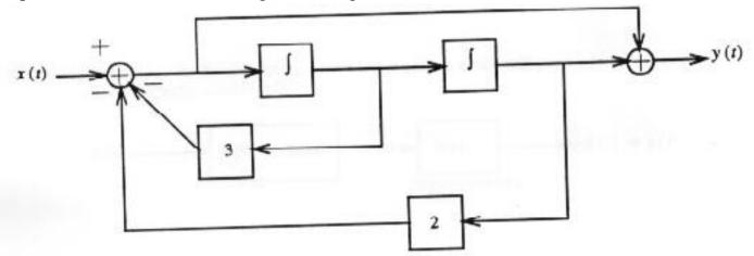
Determine the transfer function for the system: H(s) = Y(s)/X(s) =\_\_\_\_\_
