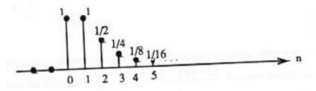
Find g[n], the impulse response of the inverse system, i.e., find a g[n] such that g[n] \* h[n] = d[n]. (Note: g[n] should be in closed form.)
