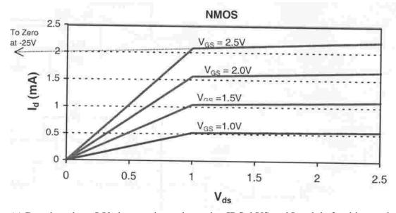
(a) Based on these I-V characteristics, determine IDS, kVS and Lambda for this transistor biased at VGS=2.5V. Put the answers in the answer boxes on page 10. (Note that the NMOS I-V equations in saturation are given on the coversheet of the exam.)
