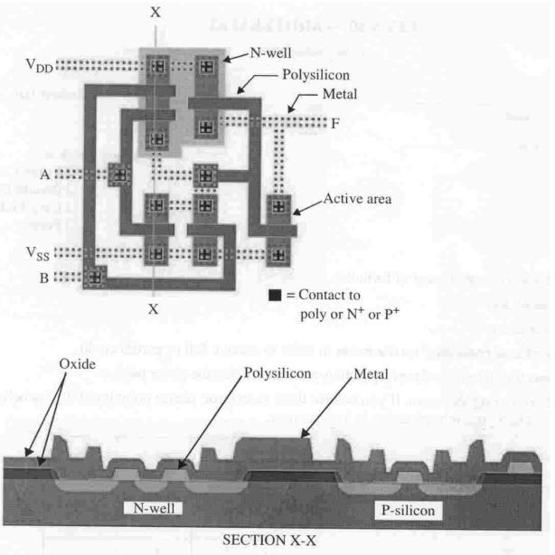
(a)Draw the circuit diagram and rearrange it to be a reasonably neat drawing. Obviously, the drawing should contain only NMOS and PMOS transistors and wires. You must, of course, label the inputs, outputs, and power supply connections.
