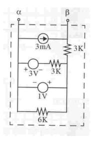
(c)Through a series of tests you find that the circuit in the box Q has thevenin equivalent shown, but you really do not know what is in the box. You now consider power flow under two conditions:
