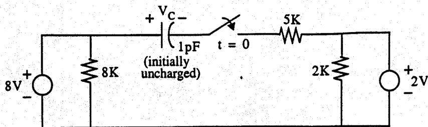
For the circuit above, the capacitor is initially uncharged. The switch closes at  $t = 0$ .
