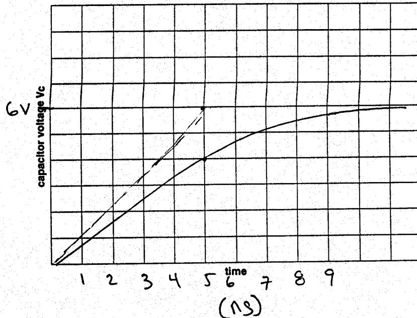
$$\text{slope at } t=0 = \frac{6\text{ V}}{5\text{ ns}}$$
