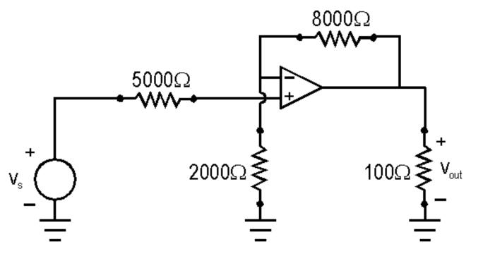
The voltage vs(t) is an endless sinusoid with frequency 1MHz and amplitude 2V, as shown here:
