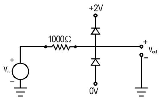
In the above circuit, the diodes are to be represented by the large signal diode model, (the one that looks like this:)
